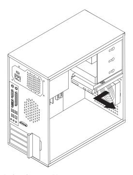
Figure 28. Removing the front fan assembly
